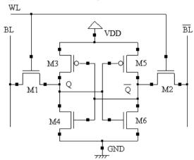
Figure 1. Conventional 6T SRAM Cell.
